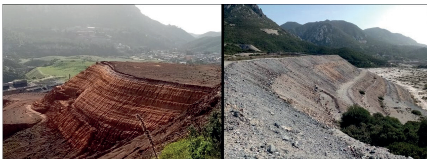
Figure 4: The “Monteponi red mud heaps”, composed of mineralogical and metallurgical processed waste (left), Sardinia - Italy. The “fine basin of Masua” comprised of tailing ponds (right), Sardinia - Italy. Source: EU Network IMPEL, Management of Mining Waste Project, 2020-2022.
